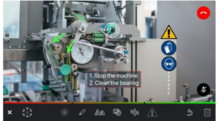
Screen capture showing notes and annotations displayed in ATS Enhanced Remote Support application.
